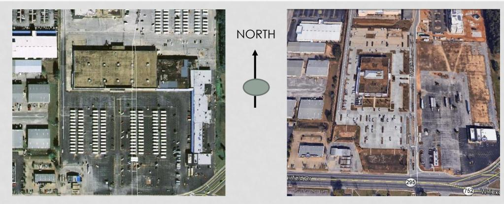
PRE (near 100% impervious) DEMONSTRATION OF STORMWATER MANAGEMENT (greenroof, pervious pavements and storage)
